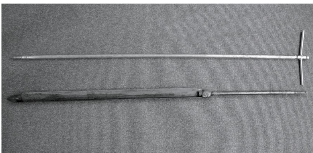
Figure 3-1. Russian peat corer, width 40 mm (bottom) and probe used for gravel/till/bedrock probing (top).
