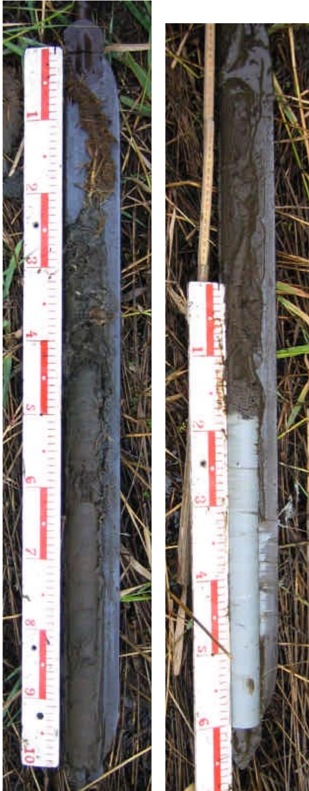
PSM006567 - "Hålö": gyttja/clay column 0–160 cm. Increasing depth down - and rightwards.
