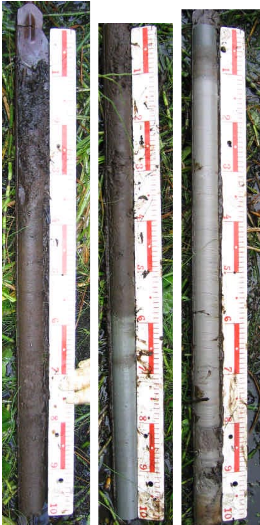
PSM006568 - "St. Ficksjön": gyttja/clay column 0–300 cm. Increasing depth down - and rightwards.
