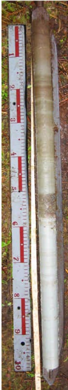
PSM006562 - "Klarebäcksmossen", peat/clay column 300–530 cm. Increasing depth down - and rightwards.
