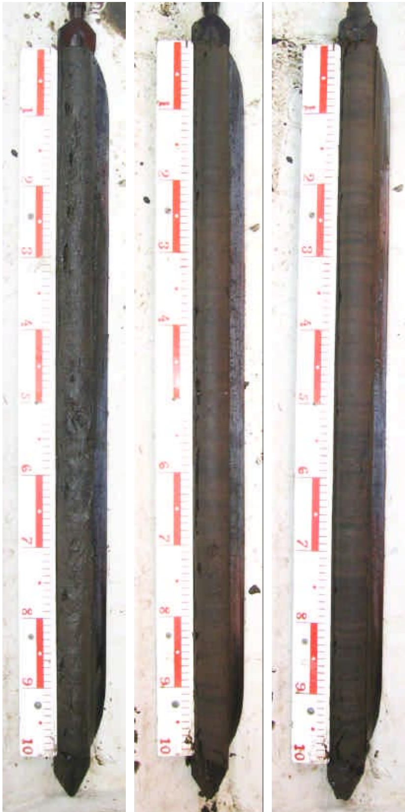
PSM006586 - "Äspö-Laxemar Bay": sediment column 0–300 cm. Increasing depth down - and rightwards.
