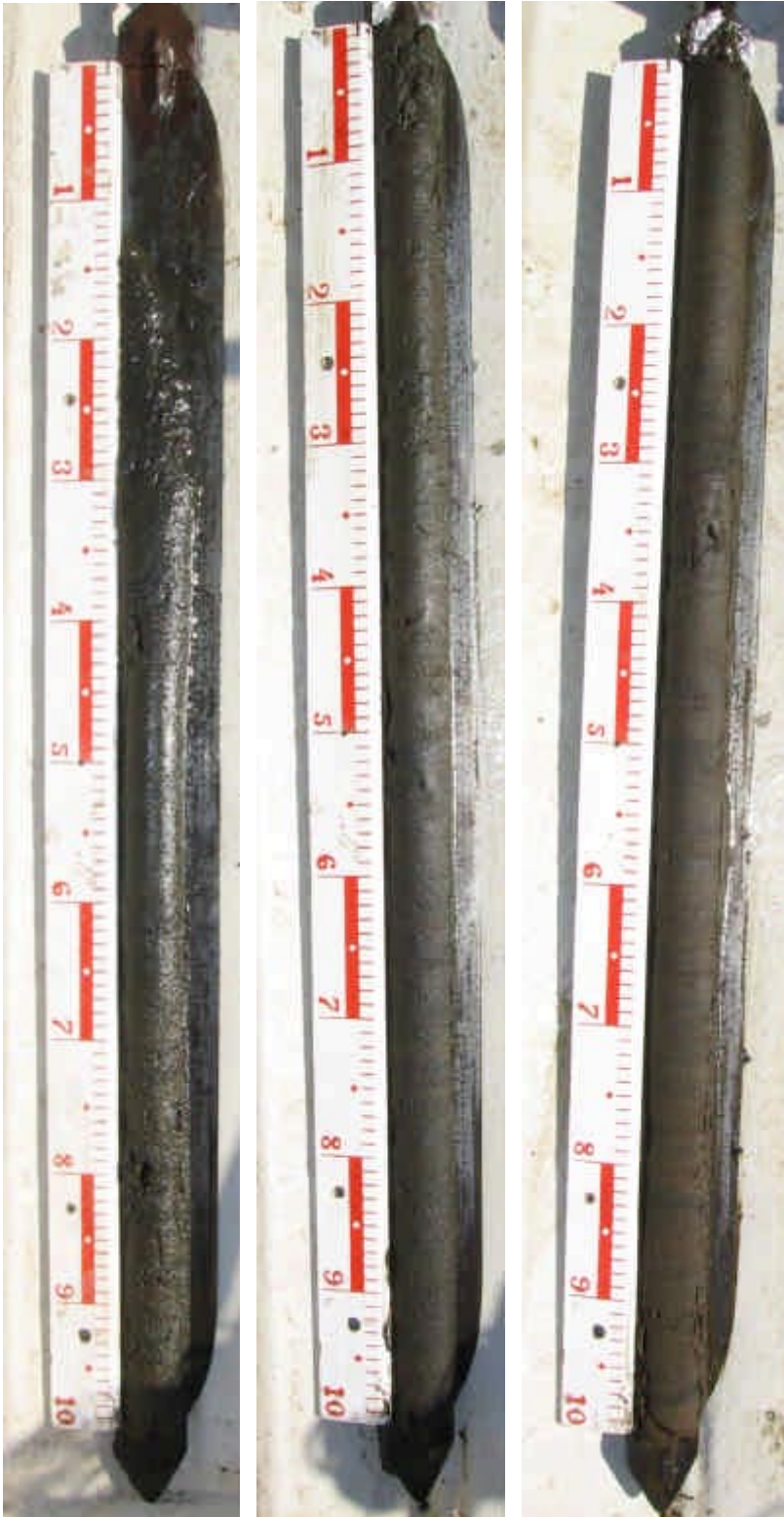
PSM006585 - "Äspö-Laxemar Bay": sediment column 0–300 cm. Increasing depth down - and rightwards.
