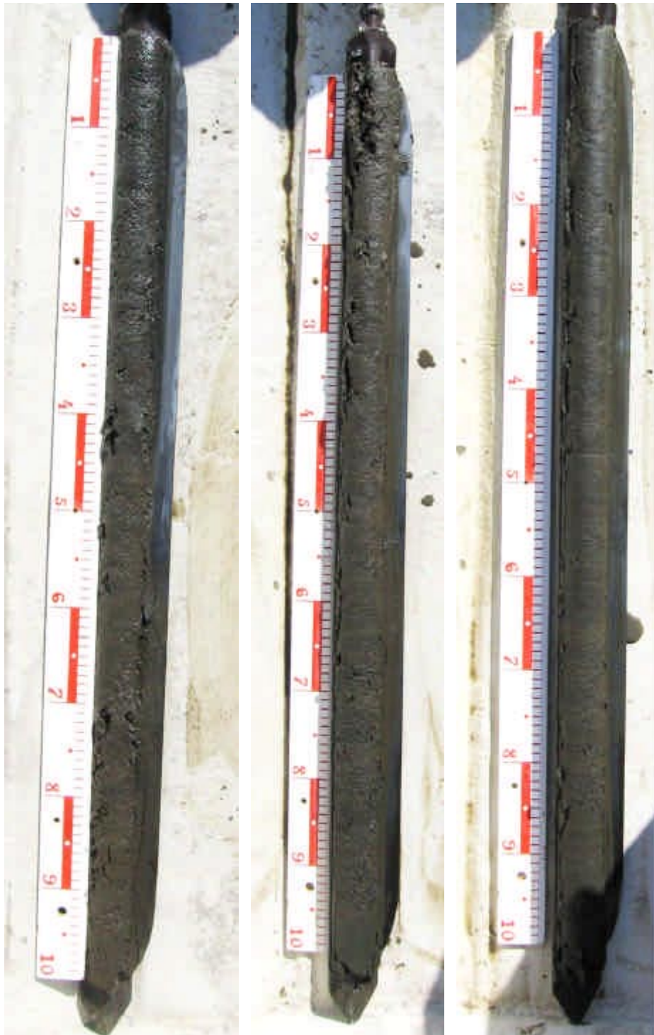
PSM006576 - "Söråmagasinet": sediment column 0–300 cm. Increasing depth down - and rightwards.
