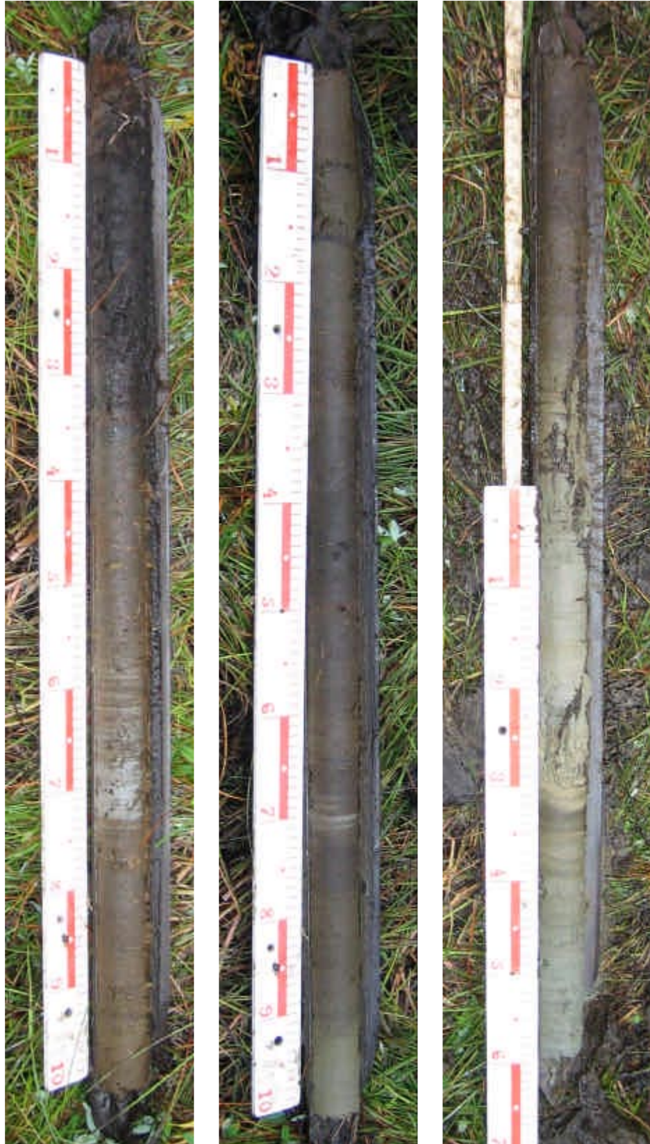
PSM006564 - "Långenmossen", peat/clay column 0–260 cm. Increasing depth down - and rightwards.
