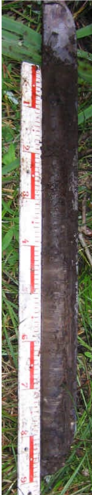
PSM006565 - "Hultenäs", gyttja /peat/ gyttja column 0–85 cm. Increasing depth down - and rightwards.
