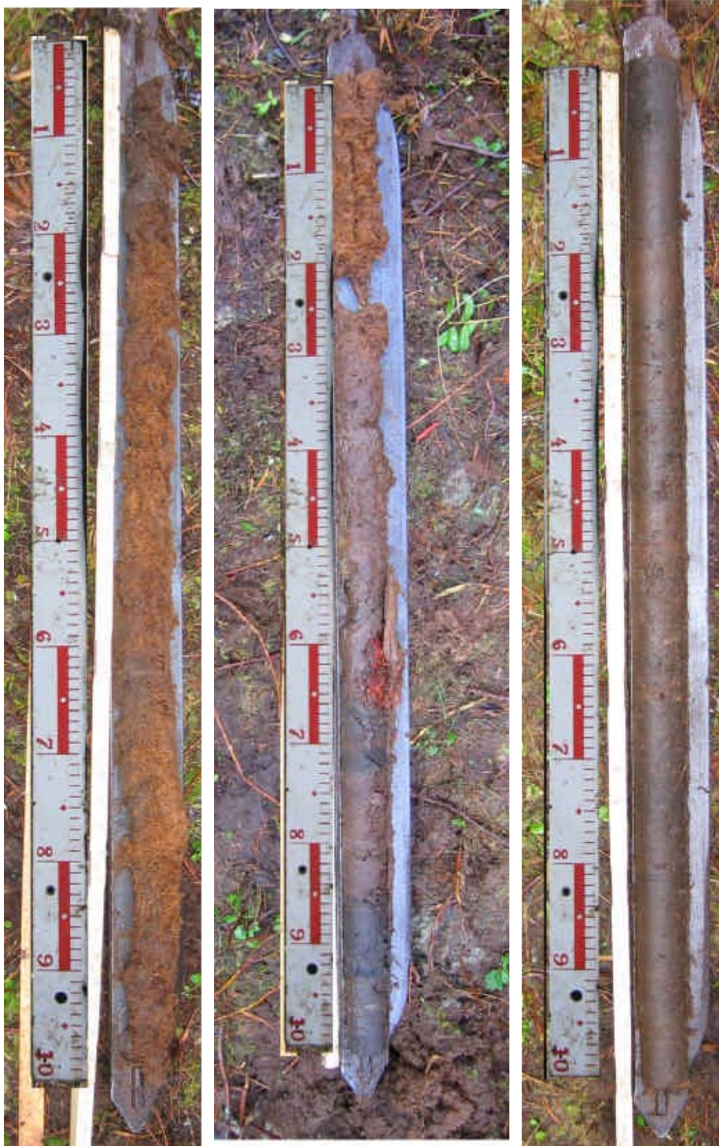
PSM006562 - "Klarebäcksmossen", peat/clay column 0–300 cm. Increasing depth down - and rightwards.
