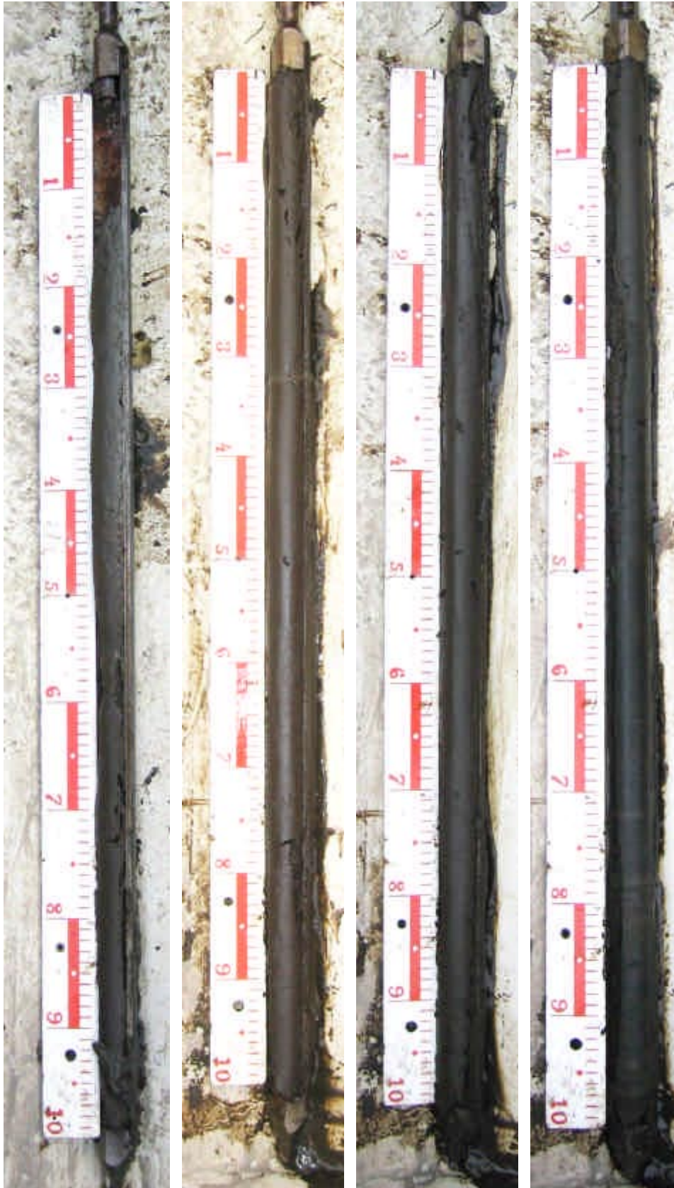
PSM006572 - "Frisksjön": sediment column 0–400 cm. Increasing depth down - and rightwards.
