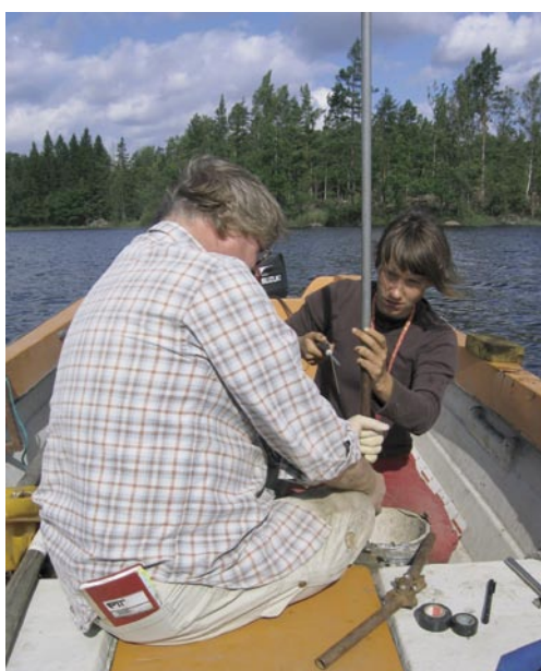
Figure 3-2. Assembling of aluminum extension rods onto the Russian peat corer.
