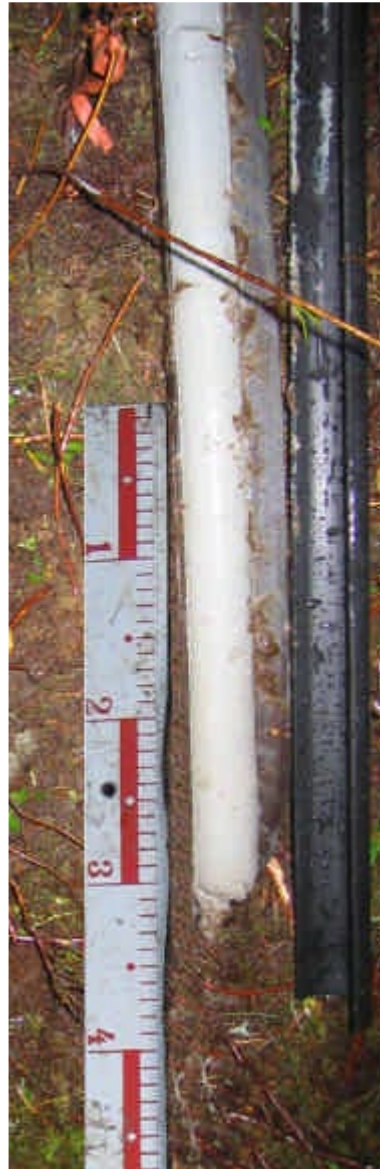
PSM006562 - "Klarebäcksmossen", peat/clay column 300–530 cm. Increasing depth down - and rightwards.
