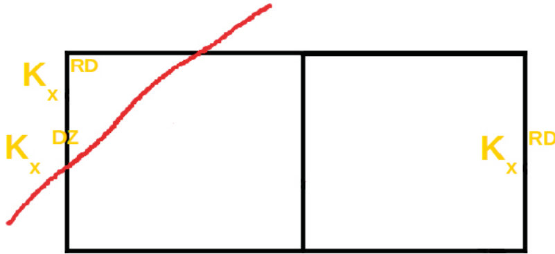
Figure 5-11. Example of equivalent hydraulic conductivity for face x using K_x^{DZ} and K_x^{RD} , for the left cell intersected by a deformation zone.
