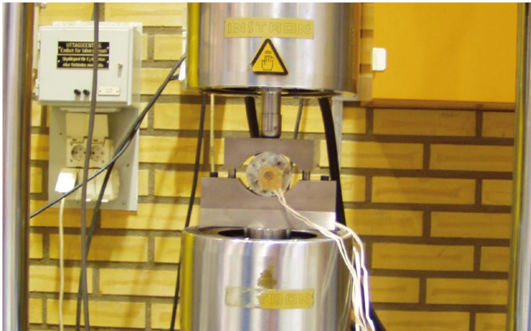
Figure 3-1. Setup for the indirect tensile test. One specimen is inserted between the curved bearing blocks, which are mounted in the testing equipment.
