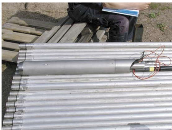
Photo 5. Positioner, bottom end of down-in-hole string.
